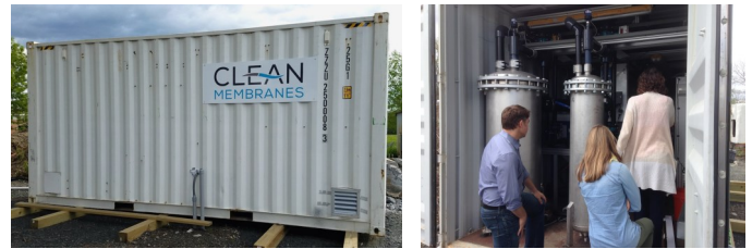
The containerized C 2 -UF WR pilot system features two compact Gigamem® modules with Neophil™/PVDF membrane fibers.
